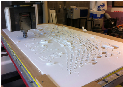
CNC Routing in Full-Scale (each component 8'x4')
